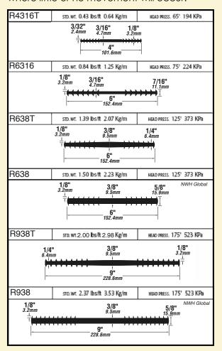
**NOTE:** The original waterstops featured a dumbbell design, but ribbed shapes provide a better seal.
