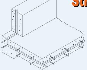
There are applications suited for easy to install, stripapplied waterstops. Typical applications include: culverts, foundations, retaining walls, slabs-on-grade, concrete pipe and pipe penetrations. These products are applied with a primer adhesive to new or existing concrete surfaces prior to a second pour. The second pour encapsulates the waterstop in the construction joint creating a barrier against fluid migration.
